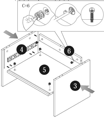
STEP 4: Insert panel (7) into grooves between panel (1) (3) (4) (5) Fix panel (1) to panel (3) (4) (6) with cam lock (C).
