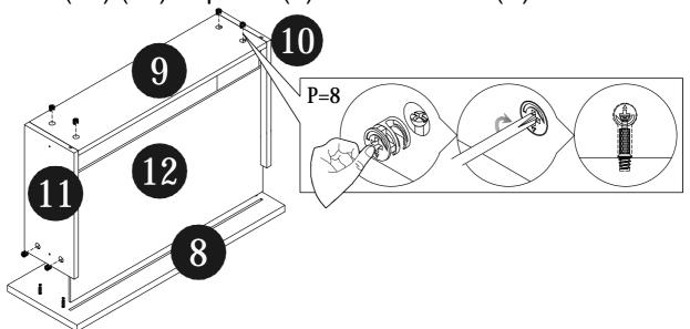
STEP 7-3:Fix rails (N-2) to panel (10) (11) with screw (V1)
